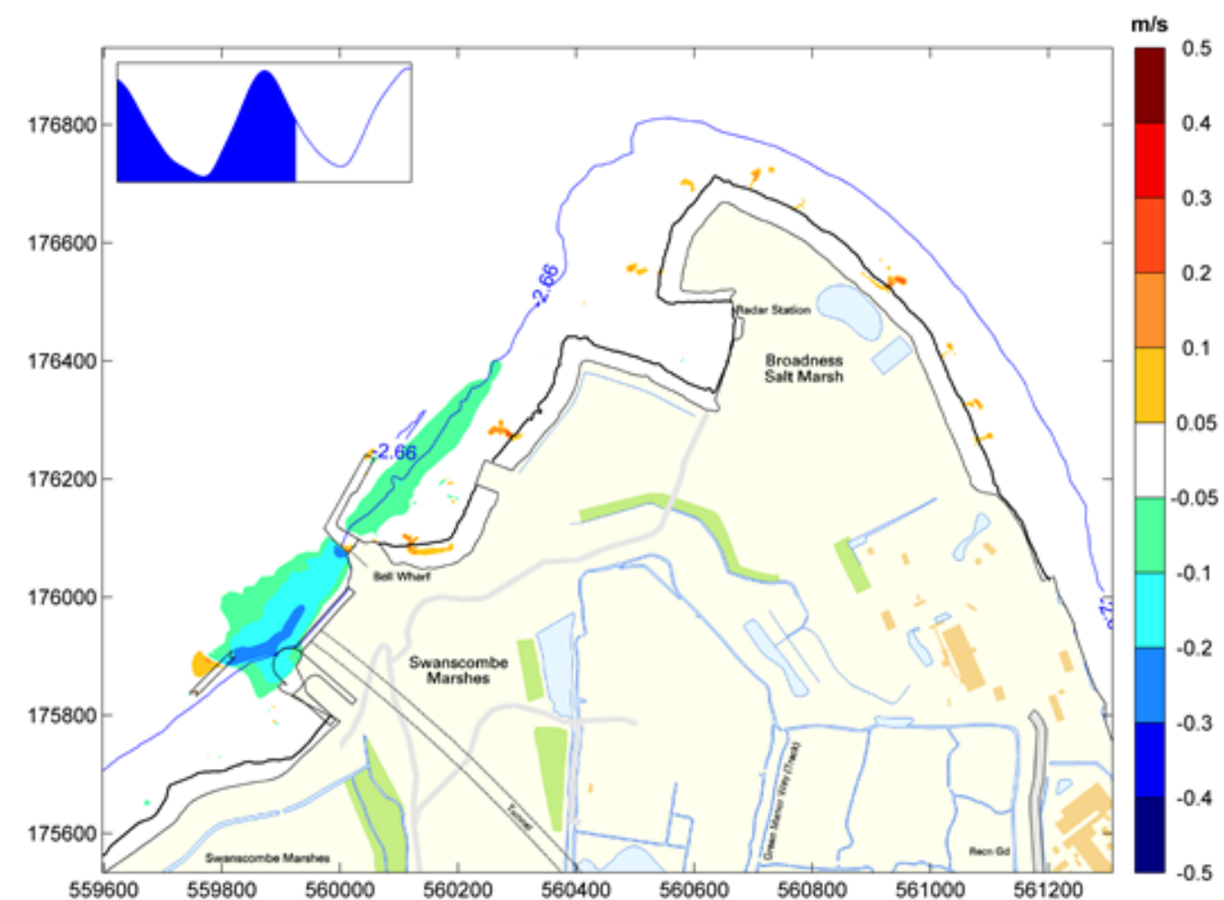
Figure 17.29: Kent Project Site Option C difference in current magnitude at time of peak ebb tide against the baseline model.
